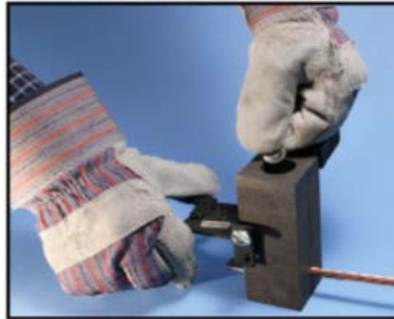
Mold being locked and disk inserted
